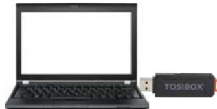
2. Open the TOSIBOX® Key software by plugging a matched Key into the USB port of your computer.
