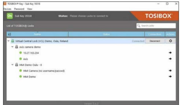
Key user interface (installed from the Key device). In the image you can see TOSIBOX® Lock devices which are matched with the TOSIBOX® Key and the network devices connected to each TOSIBOX® Lock.
