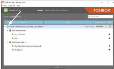
This is the start window for the Key user interface. You can open the Lock user interface by double clicking the Lock icon on the left side of the window.
