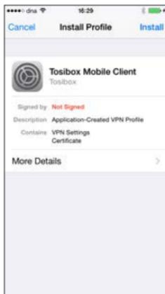
13. On the first time when connecting to a Lock, the user needs to authorize the installation of the VPN profile by entering the device passcode.
