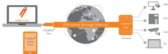
With its factory default settings, the Lock is connected to the Internet via its WAN port or a USB modem which can be connected to the USB port of the Lock. In this mode, the Lock creates its own protected local network for the connected devices. In this configuration, only devices that are connected to the Lock by cable or via WLAN access point are accessible with the Key.
