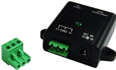
The APOE03G is the Single-Port Gigabit ( 10/100/1000 Base-T) redundant PoE Midspan/Injector that provides DC power for PoE equipped Network Appliance device. It is compatible with devices that support the IEEE 802.3af/at standard PoE power feed using Mode B (Pins 4/5 and 7/8).
