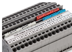
The 1-to-3 adjacent jumper for continuous commoning enables every other terminal block to be commoned. For example, positive and negative potentials can be accommodated alongside each other.
