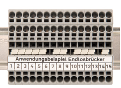
Continuous jumpers (2002 Series) readily connect an endless number of terminal blocks to each other via single jumper slot. Use the second jumper slot for additional commoning or testing.
