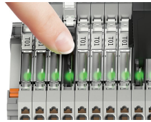
Configuration via push/slide switch
