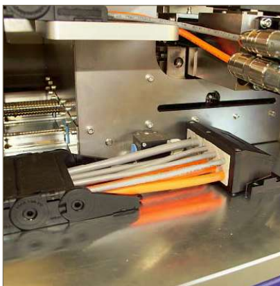
KEL-FG A10 - Page 26 In conjunction with cable carriers for strain relief and cable routing into an integrated switch cabinet.
