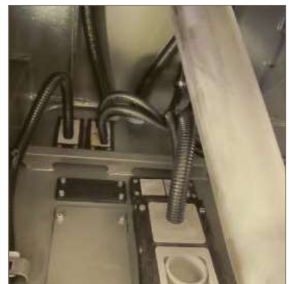
KEL-JUMBO 2 - Page 48 / KEL 24|x - Page 16 Routing of conduits and large cables in the vehicle frame.
