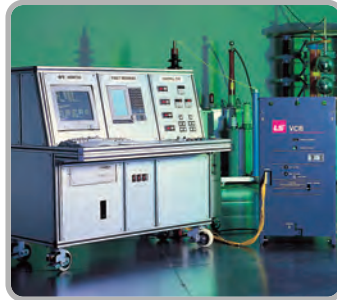
Characteristics Test / VCB Characteristics Test
