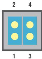
Jumpers 1 and 2 are used to enable the Ring Master
